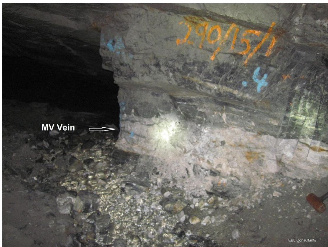
Exhibit 9 : MV low angle quartz vein (location on the 300 SB East Level at the top of stope 290-15).
